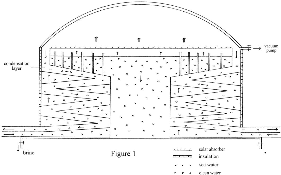
The desalination tank is circular, of diameter one kilometre and is sealed with a double glazed dome. It contains water to a depth of 10 metres and air at a pressure of 0.1 atmosphere. About one metre above the water level, there is a solar absorber covering the entire surface. This is abundantly perforated with millions of small holes to allow the upward flow of air and water vapour.
